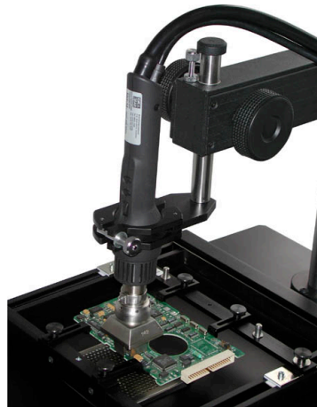
Position distance of Nozzle-to-PCB
