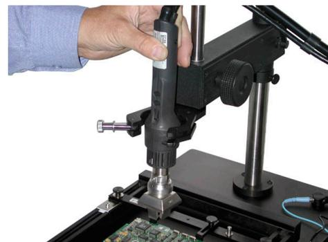
2. Place the XTH Series Tool straight in vertical position inside the clamp, matching clamp profile to the one of the handle.
