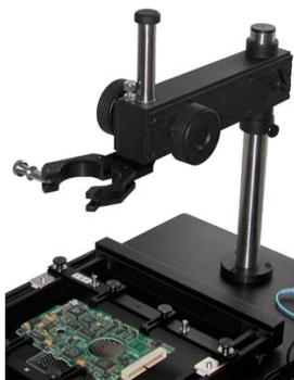
1. Turn the nut clenches arm (1) counterclockwise several turns to release the arms fasten XTH Series Tool (2). Spread the arms fasten XTH Series Tool.
