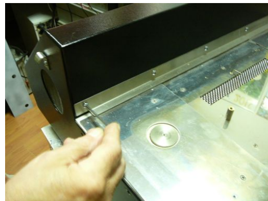
4b. Remove the front angle iron held by 5 M4 screws as shown above
