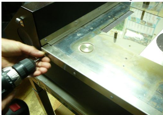
4a. Remove the angle iron held by 6 M4 screws
