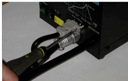
Tighten 2 screws (one on each side of a connector) using flat screwdriver to secure the connector in place
