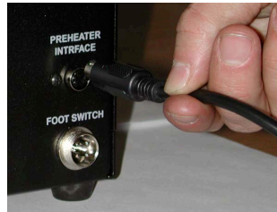
d). Tighten the nut turning it clockwise.
