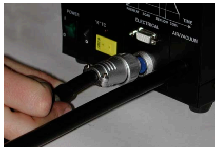
Connect round power plug to a matching socket on the unit.
