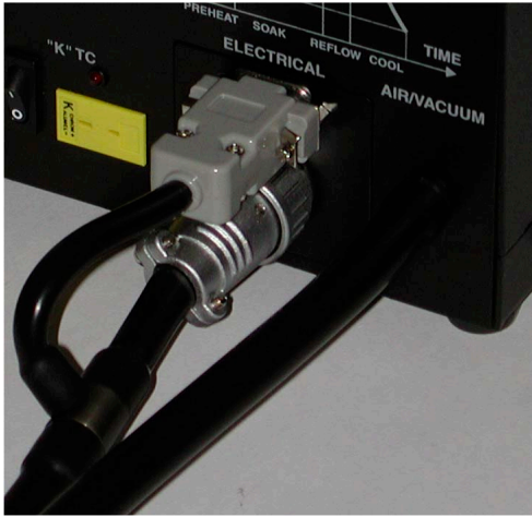
XHT-15 hand piece connected on front panel
