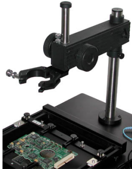
a). Turn the nut of the clamp counterclockwise to open it.
