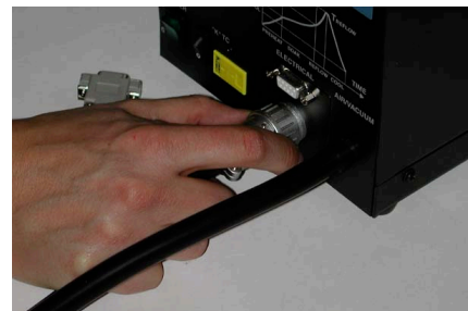
Tighten the ring to secure the connector
