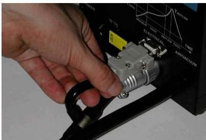
Connect multi-wire plug to a matching socket on the unit.
