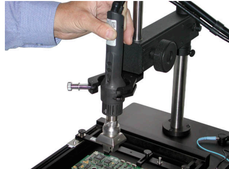
b). Place the XTH Series Tool straight in vertical position inside the clamp, matching clamp profile to the one of the handle.
