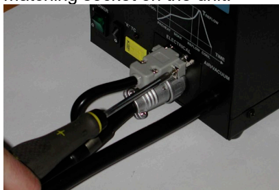
Tighten 2 screws (one on each side of a connector) using flat screwdriver to secure the connector in place
