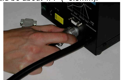
Tighten the ring to secure the connector
