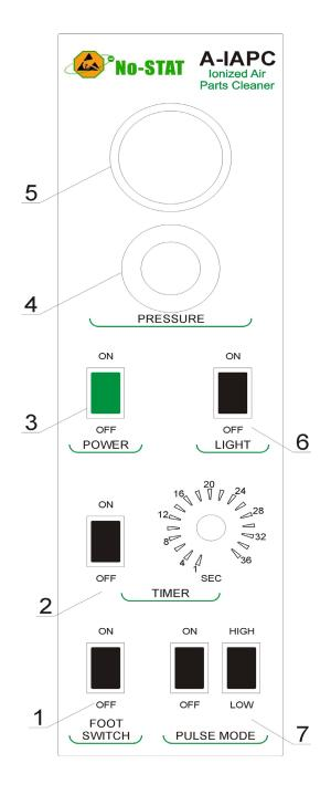
FIG. 2 VIEW OF THE CONTROL PANEL
